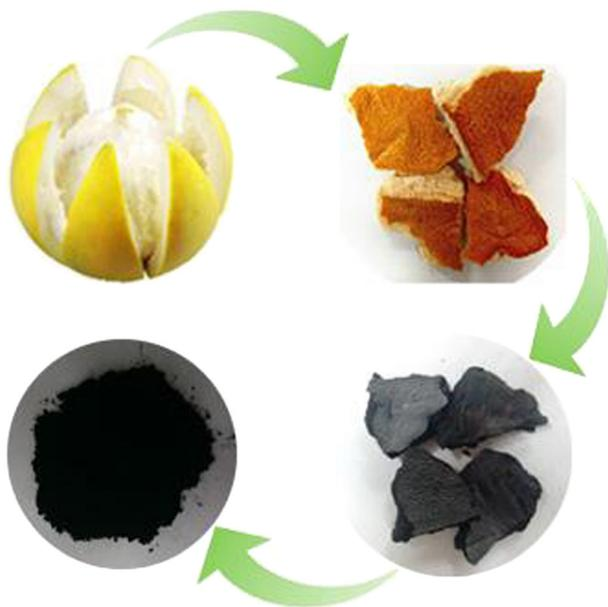
**FIGURE 1** Schematic diagram of the preparation of pomelo peel char [Colour figure can be viewed at [wileyonlinelibrary.com](http://wileyonlinelibrary.com)]
