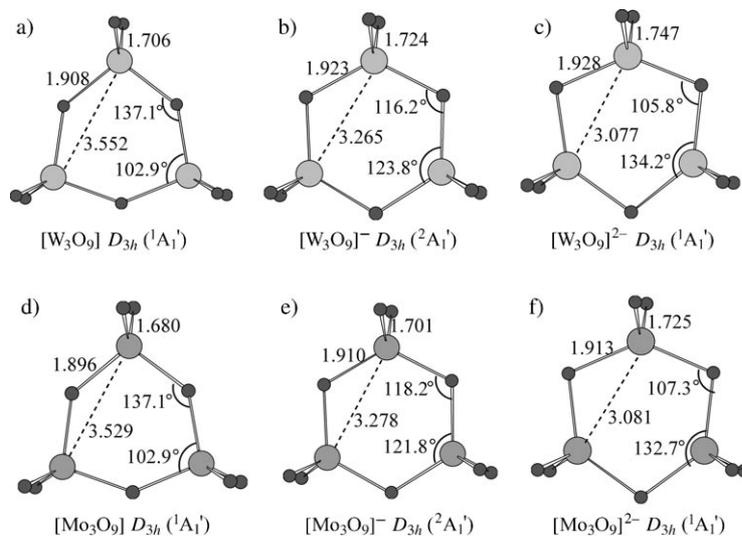
**Figure 2.** Optimized structures for [M<sub>3</sub>O<sub>9</sub>], [M<sub>3</sub>O<sub>9</sub>]<sup>−</sup>, and [M<sub>3</sub>O<sub>9</sub>]<sup>2−</sup> (M = W and Mo).
