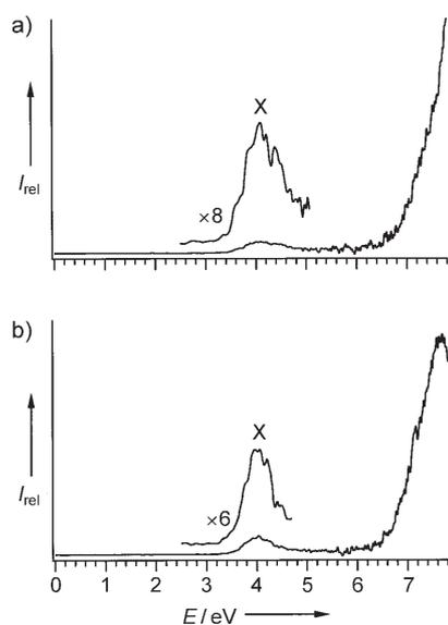
**Figure 1.** Photoelectron spectra of [W<sub>3</sub>O<sub>9</sub>]<sup>−</sup> (a) and [Mo<sub>3</sub>O<sub>9</sub>]<sup>−</sup> (b) at 157 nm (7.866 eV).
